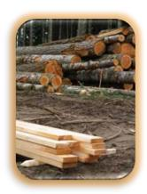
When trees are felled and brought to a lumber mill, the first step is usually to debark and sort the logs by species, size or by end use. Logs destined for wood flooring, for example, are then sawn into rough boards of the required dimensions. These are often edged or trimmed for length before they are dried.
